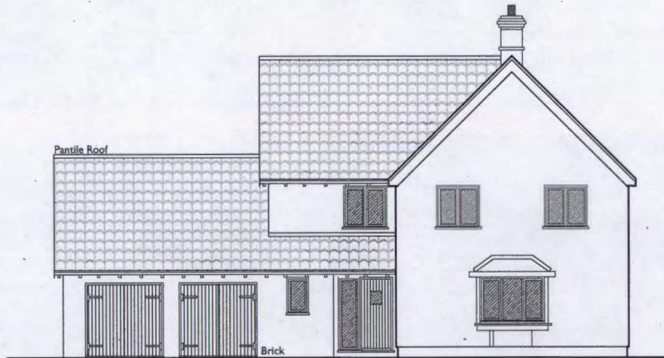
Front Elevation - North
