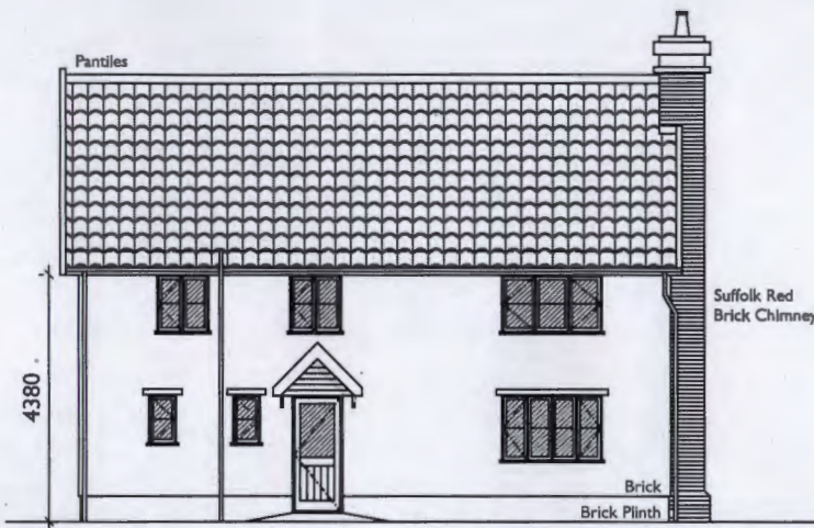
Front Elevation - North
