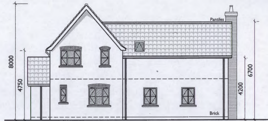
Side Elevation - North
